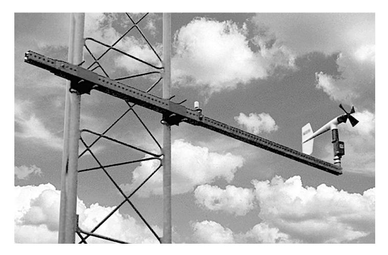
**Retractable Mounting Arm** allows rigid mounting of instruments away from tower to minimize effect of the tower structure on measurements. Tele-scopic design retracts for easy installation and service of sensor. Constructed of galvanized steel square tubing, the mounting arm is supplied with universal mounting brackets that bolt to tower legs. 1" IPS mounting post fits YOUNG sensors.
