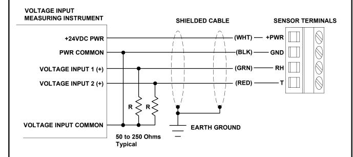
30VDC at 46 mA Max Supply Total Current Consumption = T mA + RH mA + 6 mA
